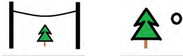
Figure 2: Vertical (Grow-in) and Horizontal (Blow-in) Conductor-to-Vegetation Gap Configurations
